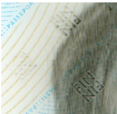
3. Embossment: micro text: "FIN", visible in sidelight and can be felt as a raised design
